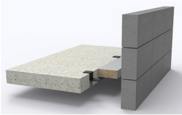
Horizontal Firestop between floor slab
